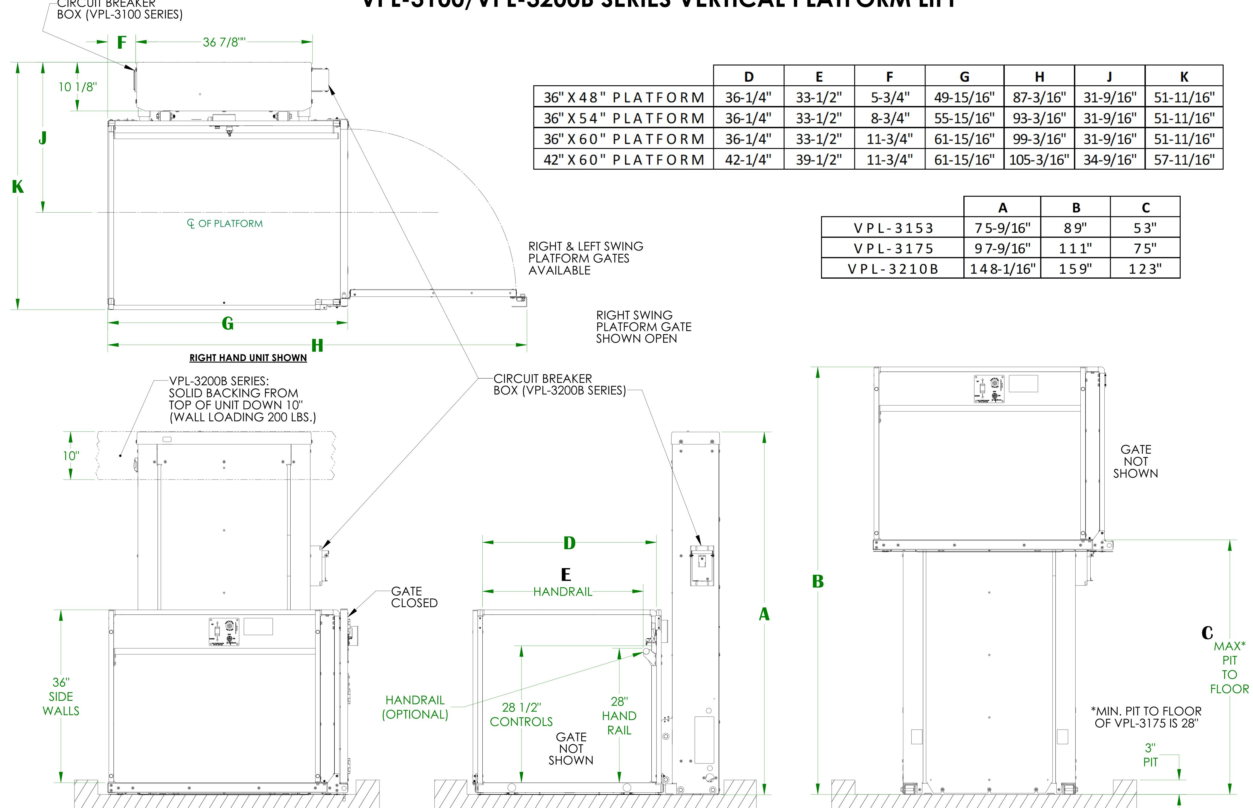
ILS-01560 SHEET 2 OF 3 REV. 0 (7683)(11/03/22)(TAK) NOTES: 1) PLATFORM GATE CAN BE MOUNTED ON EITHER SIDE OF THE PLATFORM 2) SEE ILS-01561 FOR LANDING GATE DETAIL/ALIGNMENT
