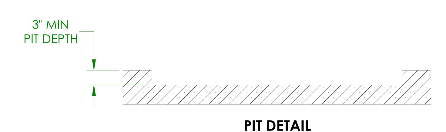
UNITS WITH STRAIGHT THROUGH PLATFORM WITH PLATFORM GATE (PIT APPLICATION)
